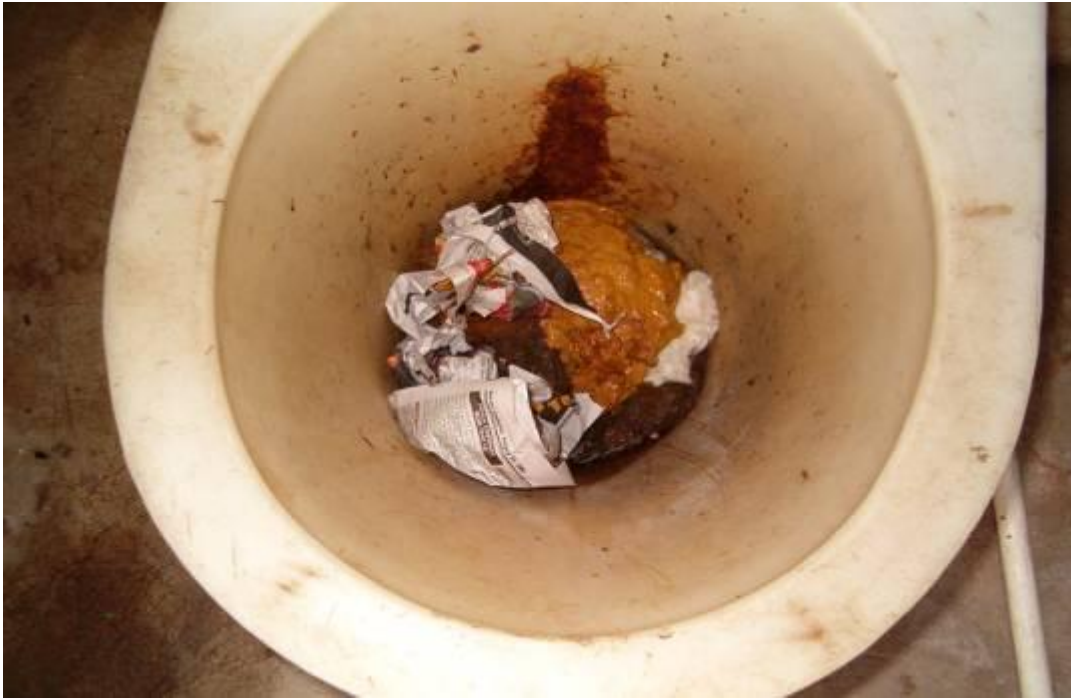
Full Pit toilet day of dosing
